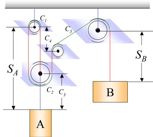
$$L = (S_A - C_3) + C_1 + (S_A - C_3) + C_2 + (S_A - C_3 - C_4) + C_5 + S_B$$
